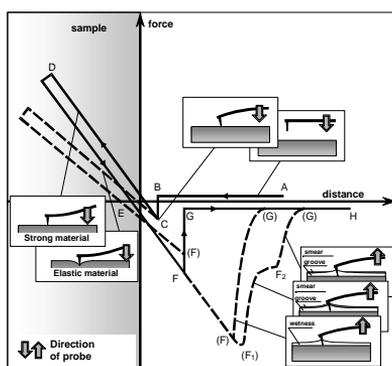
Figure 2. Nomogram of the curves - approach/ moving off. The solid lines are schematic presentation of curves obtained in vacuum. Dashed lines show variations of curves of approach/moving off conditioned by elastic features of the sample and by presence of surface layers of moisture and streaks (impurities).
