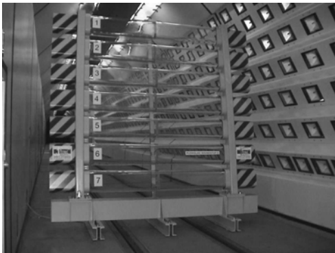
Figure 2. The prototype of the barrier in the wind channel
