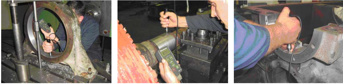
Figure 4. Measuring hardness of details after welding repair
