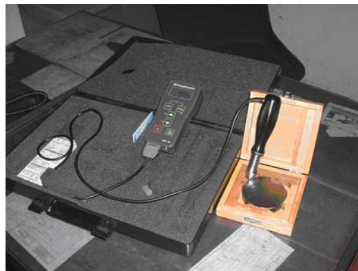
Figure 3. Krautkramer MIC 10 Unit for measurement hardness.
