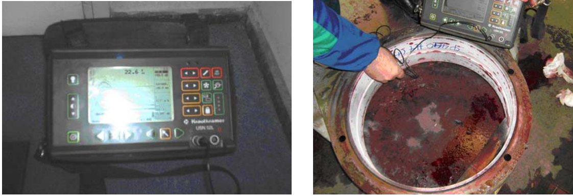
Figure 5. Ultrasound KRAUTKRAMER USN 52 L used by the Institute "INKOS" and ways of controlling the details with it
