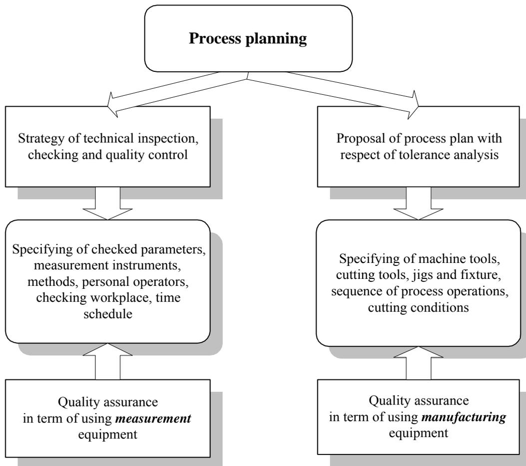
*Figure 1: Measurement and manufacturing aspect in process planning*
