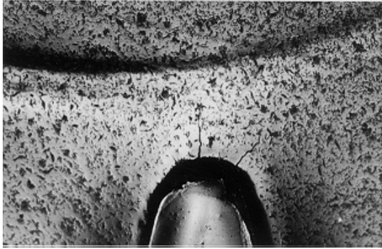
FIGURE 3. ACTIVE WORKING SURFACE OF THE DIE. SURFACE CRACKS AND PITS. MAGN. 50X.
